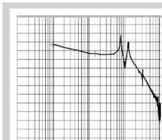
Bode diagram of an unloaded, unregulated system with two resonance frequencies.
