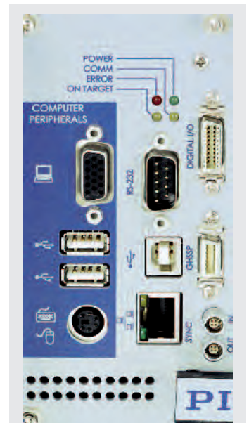
The E-712 provides RS-232, USB and RS-232 as standard interfaces. Additionally, digital I/O lines and optional analog interfaces or a real-time PIO are available.
