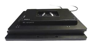
PInano™ XYZ piezo scanner mounted on a M-545.2P long travel, ultrasonic motor microscope stage. The XYZ piezo nanopositioning stages provide <1 nm resolution and are available with up to 200µm scanning range. The high stability and autolocking feature of M-545 provides significant advantages over other microscope stage designs when using fast piezo scanning stages. Request paper on long term stability!
